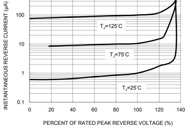
FIG. 2 TYPICAL REVERSE CHARACTERISTICS
