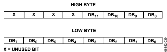
Figure 38. Data Format for AD5341
