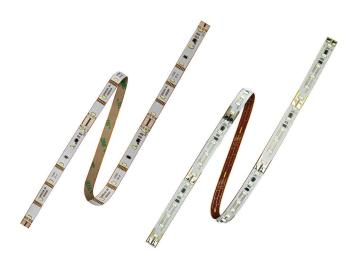
The LINEARlight FLEX LED linear modules, offered in 2700K, 3000K and 4000K color temperatures, have a color variation within a 3-step MacAdam ellipse and a CRI of >80. At 32.8 feet, the Advanced Family has a lumen output of 119 to 129 per foot with an efficiency of 81-88 LPW. The Advanced Family has the ability to support sections as short as 4 inches (6 LEDs) and to cut at every one to two LEDs at designated cut points.
