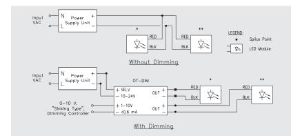
The maximum operable length on a single feed is 1 full reel.Remaining load must be connected on subsequent power feeds.Reference the "Power Supply Information" section of this PIB for module load per power supply requirements.To help reduce the effects of any potential voltage drop, if possible, it is best to locate the power supply near the middle of the run.
