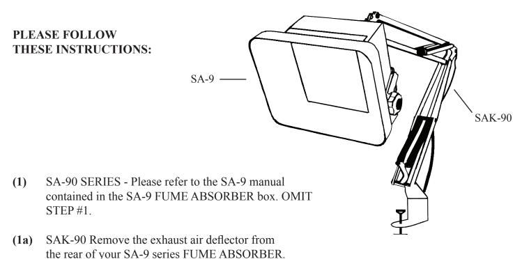
(2) Using the thumb-screws provided with the SA-9 mount the SA-9 to the "U" shaped bracket.
