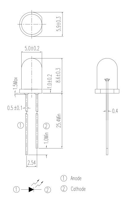
Note: Tolerances unless dimensions ±0.25mm
