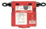
2CPS Series, Cable Pull Safety Switch, Cable, Maintained Both Sides, 2NC/2NO Direct Opening (Switch 2, Left: 1NC/1NO; Switch 2, Right: 1NC/1NO), 1/2 NPT, Gold-plated Contacts
