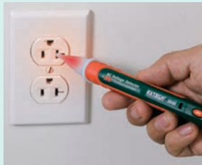
Quickly check for the presence of live wires before testing
