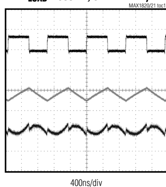
MEDIUM-LOAD SWITCHING WAVEFORMS ( V_{IN} = 3.8\text{V} , V_{OUT} = 1.8\text{V} , I_{LOAD} = 300\text{mA} , SKIP = BATT )
