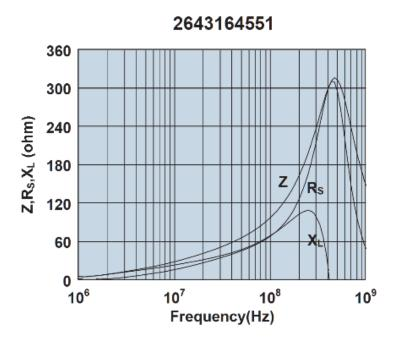
Impedance, reactance, and resistance vs. frequency.
