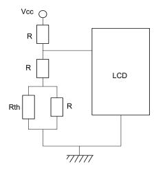
Temperature compensation (RF circuit)
