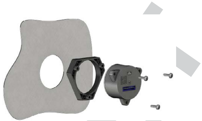
Mounting of the Design-In-Kit using the mounting ring (with double-sided adhesive tape)
