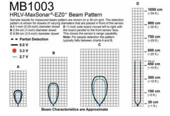
The different HRLV models have different beam width patterns, check this image for a comparison of all the HRLV model beam patterns. If you don't need high sensitivity, or want a longer range, check out the LV models - They are meant for up to 6.5 meter distances
