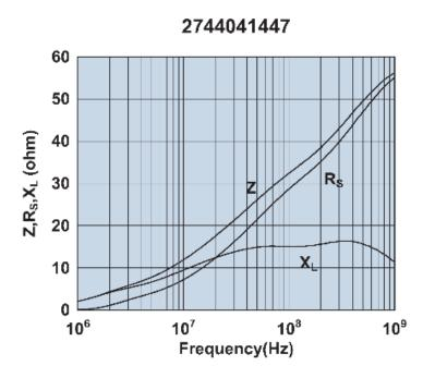
Impedance, reactance, and resistance vs. frequency.
