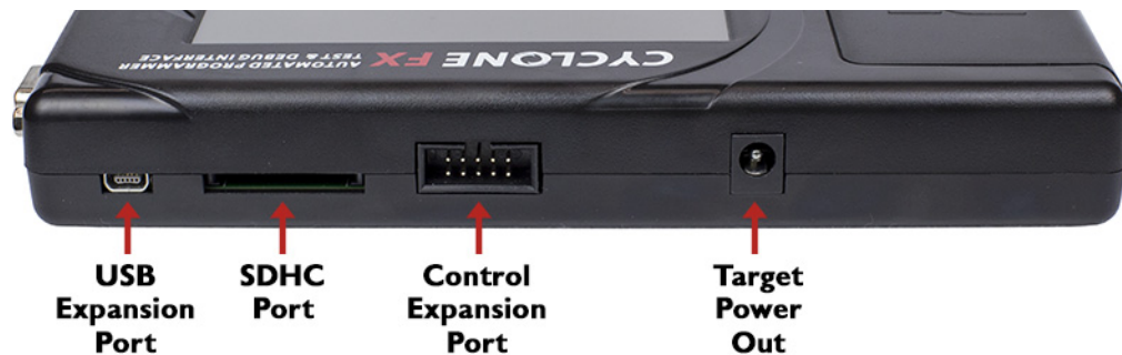
Figure 3-4: CYCLONE FX Rear Side View
