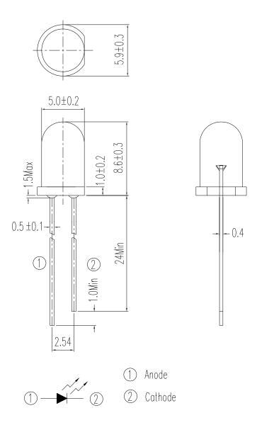
Note: Tolerances unless dimensions ±0.25mm
