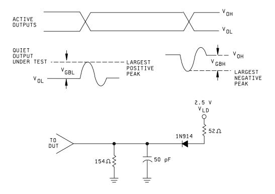
NOTE: Resistor and capacitor tolerances =  $\pm 10\%$ .
