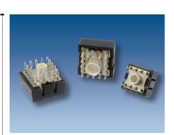
The RADSOK® PowerBlok™'s compact footprint  $\frac{1}{2}$ " x  $\frac{1}{2}$ " can supply up to 70A to backplane power connections. Current is distributed over 16 compliant pins. The PowerBlok™ is available for top or bottom entry and offered with a touch-proof cover.
