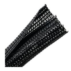
Center-slit overlapping design allows quick and easy access to the wires and cables for future maintenance or inspection without disassembly. Flexible material allows it to easily wrap around a variety of component shapes and sizes, making it easier to use than slit-loom tubing or spiral-wrap materials.
