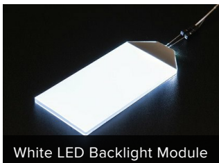
White LED Backlight Module
