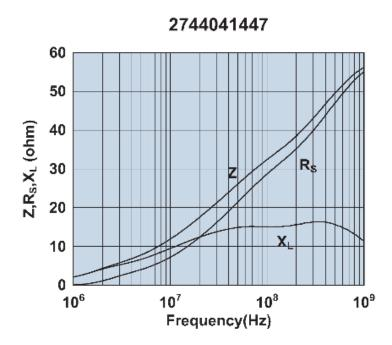
Impedance, reactance, and resistance vs. frequency.
