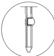
Board Retention using Swaged Tails (All Header Sizes)
