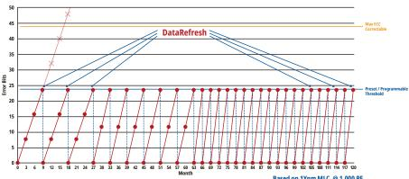
IntelligentScan/DataRefresh to proactively extend Data **Retention beyond the typical NAND flash limitation** Not to scale, for illustration purpose
