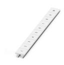
Zack marker strip, Strip, white, labeled, can be labeled with: CMS-P1-PLOTTER, printed horizontally: consecutive numbers 1 ... 10, 11 ... 20, etc. up to 91 ... 100, mounting type: snapped, for terminal block width: 10.2 mm, lettering field size:  $10.15 \times 10.5$  mm, Number of individual labels: 10
