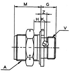
For contact data see Catalog 12-020. All lockwire holes .045 Dia. Min.
