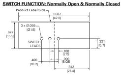
PCB Layout for LST Terminations (Unit: Inch [mm])
