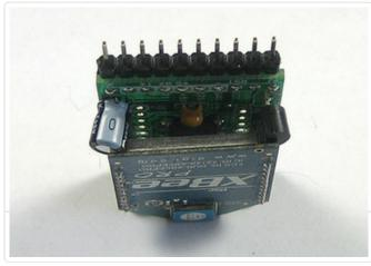
Now solder in the power supply components & clip the leads.
