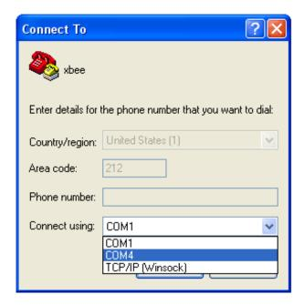
Next, set the properties. Make sure you select **9600 bps, 8 bit, No parity, 1 stop bit and no flow control.** Some programs may call this (9600 8N1). If the XBee has been configured for a different baud rate, of course, you should use that.
