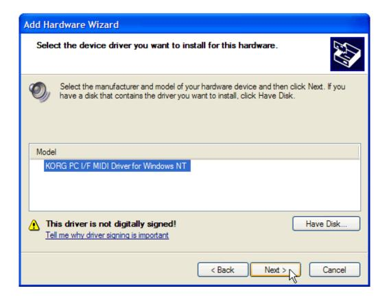
Make sure the FTDI cable is set to COM2, 3 or 4 because the driver can't cope with higher numbers. You can set the FTDI cable's COM port in the Device Manager. Set the KORG driver to the correct COM port.
