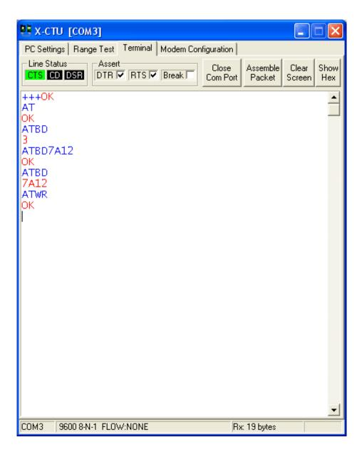
OK now you have set the XBee to 31250 communication. You can hard reset the XBee by un/replugging the adapter. Test that you did things right by trying to connect to the XBee again, now at 31250. Remember that you have to select 38400 as the connection baud rate because that is *aliased* to 31250.
