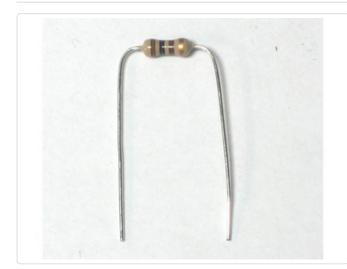
First thing we will place is **R3**, a 10K resistor (brown, black, orange gold). This resistor is used to keep the XBee out of reset mode, so that by default it is on.
