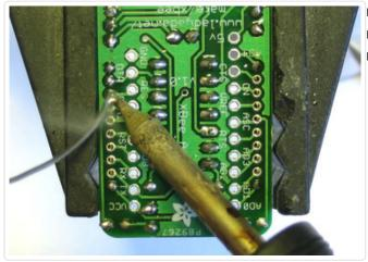
may 'fill' with solder. Use only the minimum necessary! If you use too much, use solder wick to remove some solder
