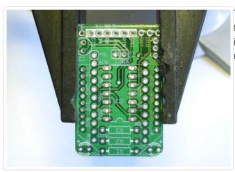
To begin, place the PCB in a vise or third-hand so that it will be easy to work on. Heat up the soldering iron to 700degF and get all the parts and tools ready for use.
