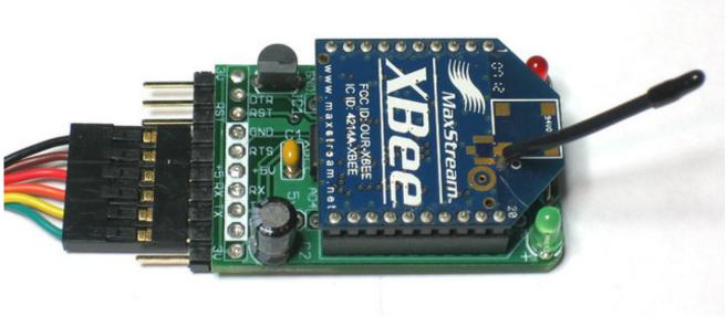
Another method of connecting is using a USB or serial breakout board. Each breakout board is going to be a little different so check the documentation. Make sure the transmit/receive pins are not swapped, etc.
