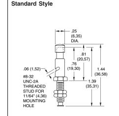
Red/Black cap Part No. 29-100 No cap Part No. 29-110 No cap, high temp. Part No. 29-125
