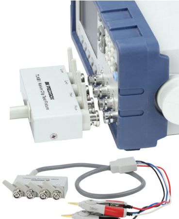
Kelvin clip test fixture
