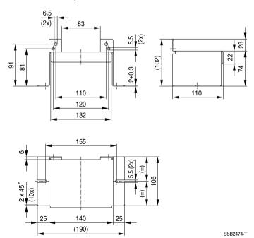
General tolerances according to ISO 2768-cL Dimensions in mm
