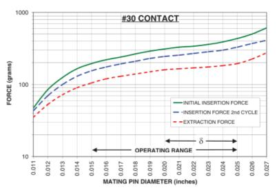
The insertion / extraction force characteristics above were derived using a 30 microinch gold-plated contact and polished steel gauge pins having a bullet-shaped tip. The curves represent typical average values; they are best used to compare the differences between similar size contacts and to guide you in selecting one that is suitable for your application. Your results may vary, so for your specification, we encourage you to obtain complimentary samples for your evaluation.
