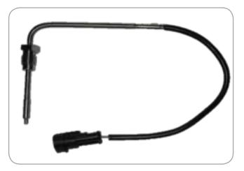
This sensor operates over a temperature range from -40 °C to 850°C. It monitors the temperature before and after SCR system in the diesel engines as part of the engine control strategy. It is designed for fast response, optimized for thermal dissipation and suitable for high vibration and corrosive environments.
