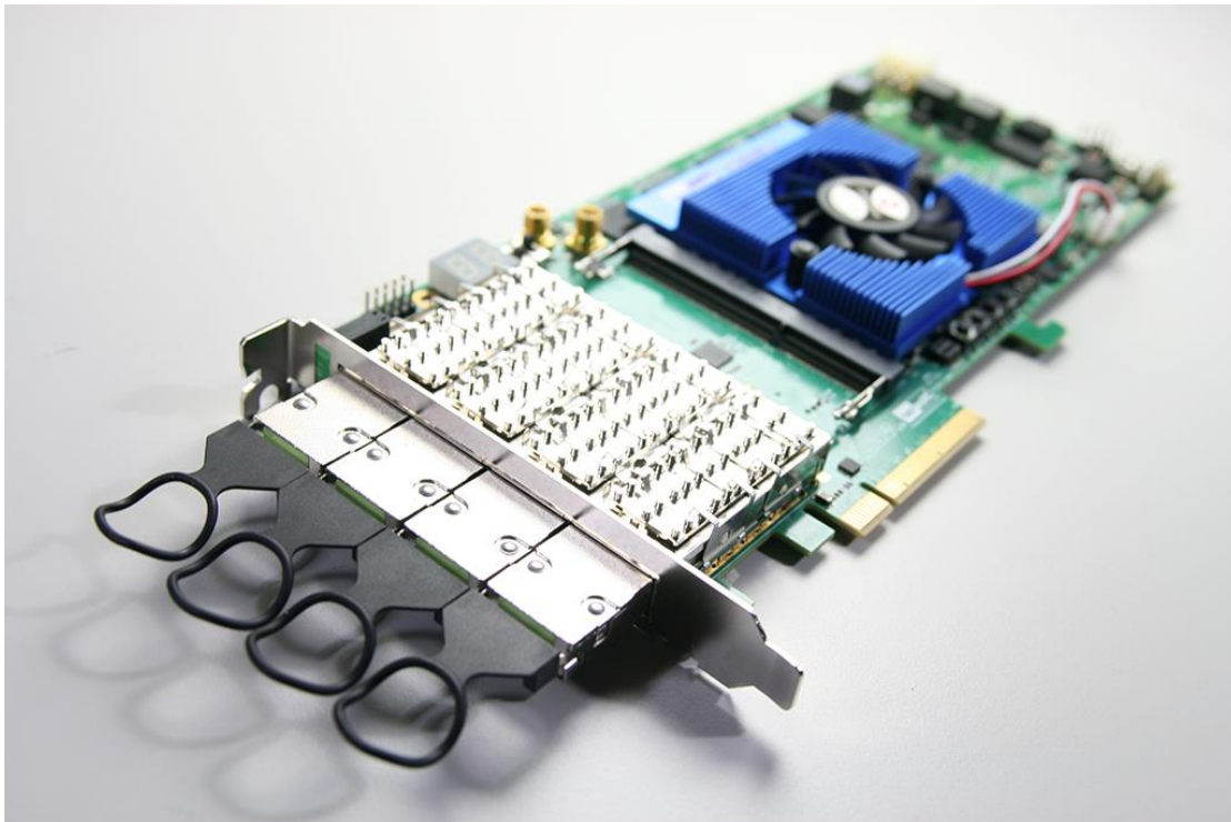
Figure 8-4 Four QSFP+ Loopback Fixtures Installed
