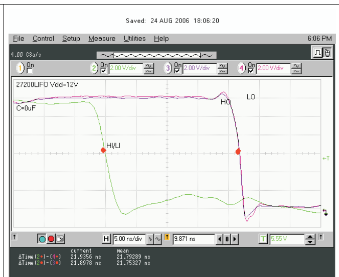
Figure 31. V_{LO} and V_{HO} Falling Edge Delay Matching
