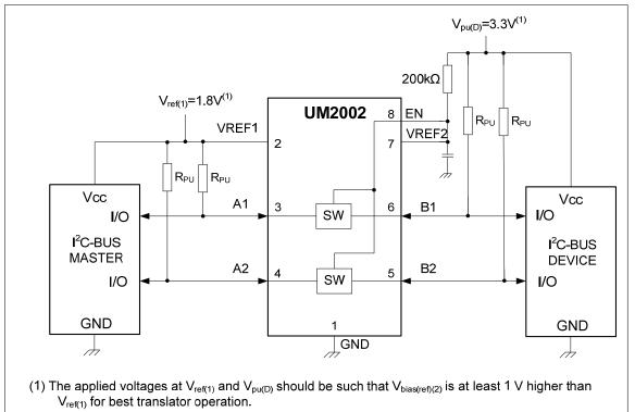
Fig 2. Typical application circuit (switch always enabled)
