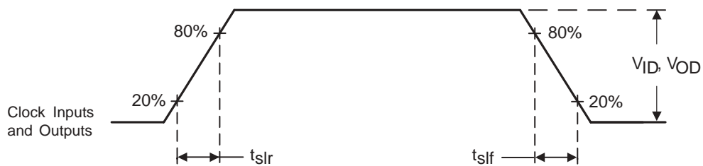
Figure 8. Input and Output Slew Rates
