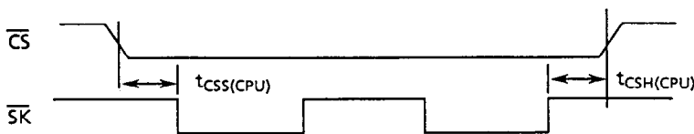
Figure 4 Timing chart of t_{\text{CSS(CPU)}} and t_{\text{CSH(CPU)}} when connected to CPU
