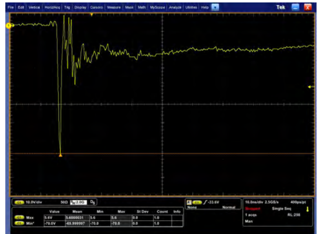
Figure 2. ESD Clamping Voltage Screenshot Negative 8 kV Contact per IEC61000-4-2
