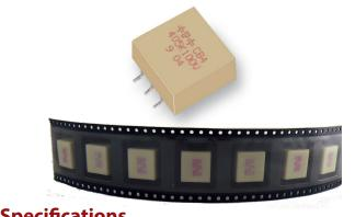
The CB style capstick capacitor is constructed non-inductively with metallized polyester dielectric. The low inductance and low ESR construction makes it ideal for high frequency switching power supplies. CB type capacitors can be used with pick and place assembly and the -FS parts are fully RoHS compliant and capable of high temperature lead free soldering.
