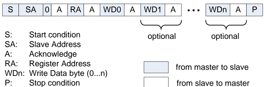
Figure 55 I2C write
