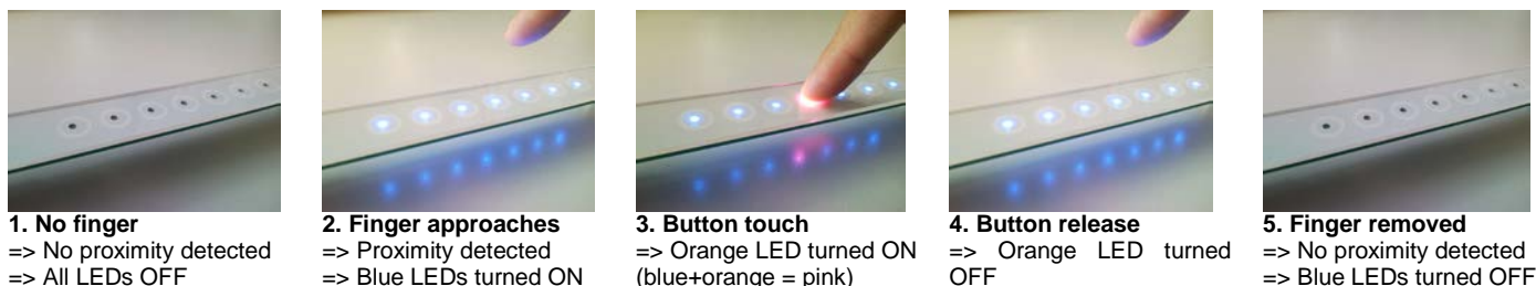
Figure 63 Touch+Proximity Module Operation
