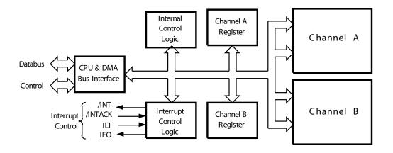
Figure 1. Z85233 Functional Block Diagram
