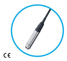
The ILSU is designed for use in continuous submersion in liquids such as water, oil and other non-aggressive chemicals. The submersible uses the latest piezo-resistive media-isolated silicon sensing technology and a stainless steel diaphragm within a 316L stainless steel housing.
