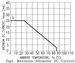
Fig4. Maximun Allowable DC Current vs. Ambient Temperature
