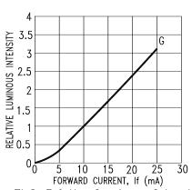
Fig3. Relative Luminous Intensity vs. DC Forward Current
