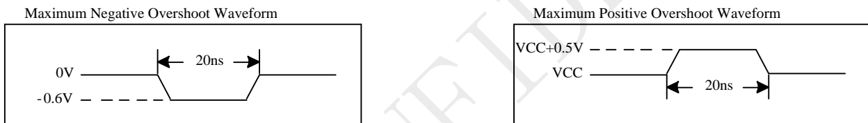
Figure 5-1 Maximum Overshoot Waveform
