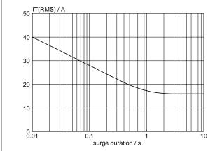
Fig.5. Maximum permissible repetitive rms on-state current  $I_{T(RMS)}$ , versus surge duration, for sinusoidal currents, f = 50 Hz;  $T_{hs} \le 38$  °C.
