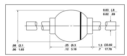
FIG. 106: Axial Lead Rectifier Outlines
