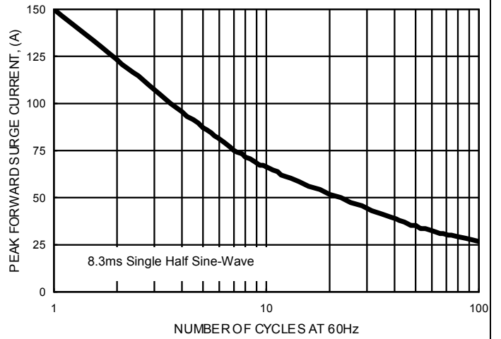
FIG.2- MAXIMUM NON-REPETITIVE SURGE CURRENT
