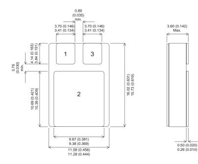
Bipolar PNP Device in a Hermetically sealed Ceramic Surface Mount Package for High Reliability Applications
