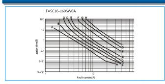
I trip= Trip current: minimum current at which the device will always at 25°C still air.
