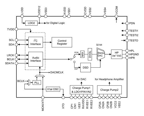
Figure 1. AK4377 Block Diagram
