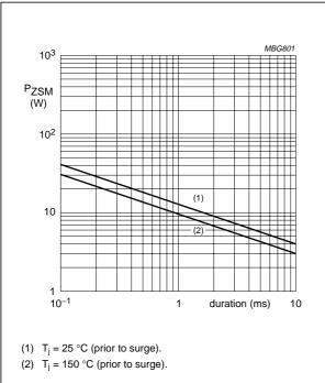
Fig.2 Maximum permissible non-repetitive peak reverse power dissipation versus duration.
